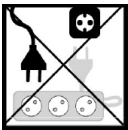
If an extension lead may become overloaded
