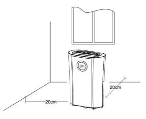
the dehumidifier should be positioned in a central and clear location so that it can draw this moist air towards it from all over the home. A warm hallway or landing is an excellent position for your dehumidifier. If possible, leave interior doors ajar to allow air circulation.
