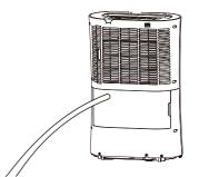
Make sure the connection between pipe and the drain outlet is tight and does not leak. Then direct the pipe to a suitable drainage point. This unit uses gravity fall to dispose water hence the drain should be lower than the unit water outlet. Put the tank back. Be sure to run the water pipe downward and let the water to flow out smoothly. Do not kink or bend the pipe.
